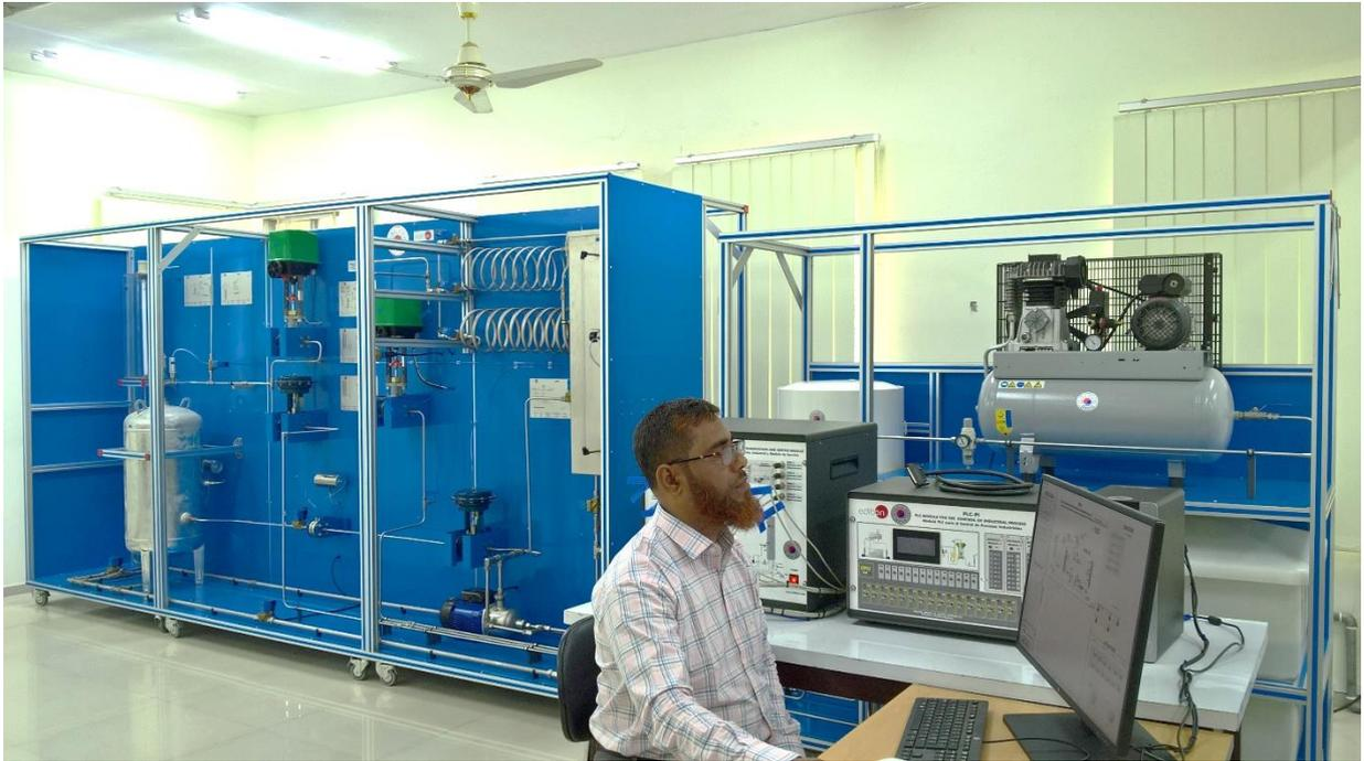
Fig: Process Control Plant with SCADA & PID control
