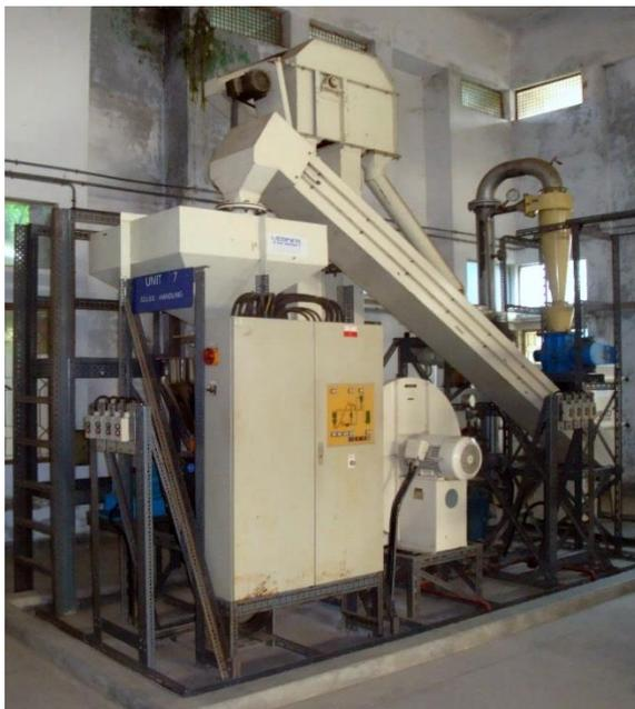
Fig: Solid Handling Unit Operation Plant
