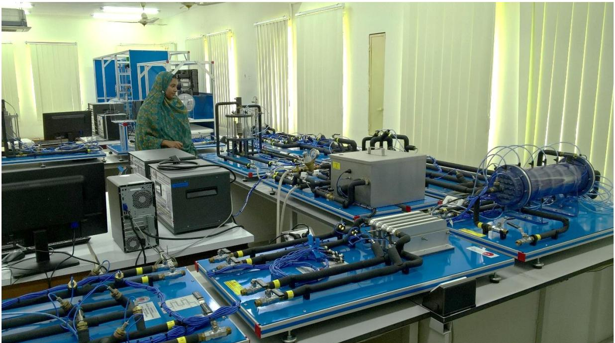
Fig: Heat Exchange Training System with SCADA and PID Control
