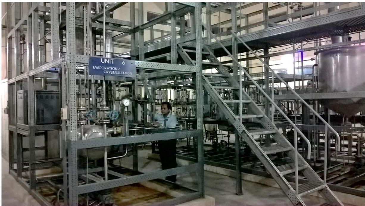
**Evaporation-Crystallization Pilot Plant:** The above pilot plant hooked-up together with Absorption/Neutralization Pilot Plant to constitute Ammonium Sulphate production system. Trainees face a critical drawing and designing environment to work in a three floored area. Moreover, an open view of crystallization and centrifuging give them an esteem knowledge on granulation system.
