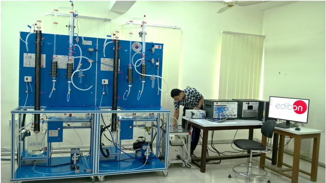
Fig: Double Effect Rising Film Evaporator with SCADA and PID Control
