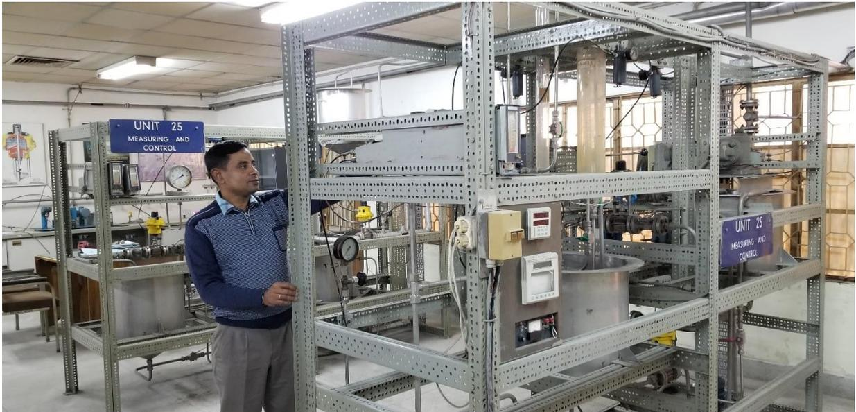
Fig: Study of Process response & Control mode in automated level control loop
