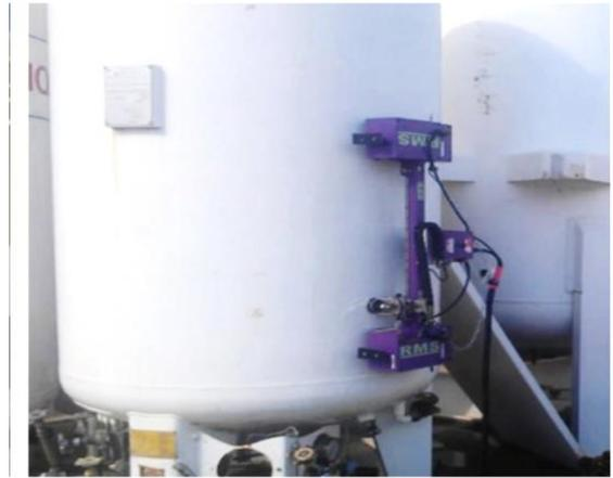
Fig: RMS2 450 for Tank & Pipeline corrosion testing and profiling
