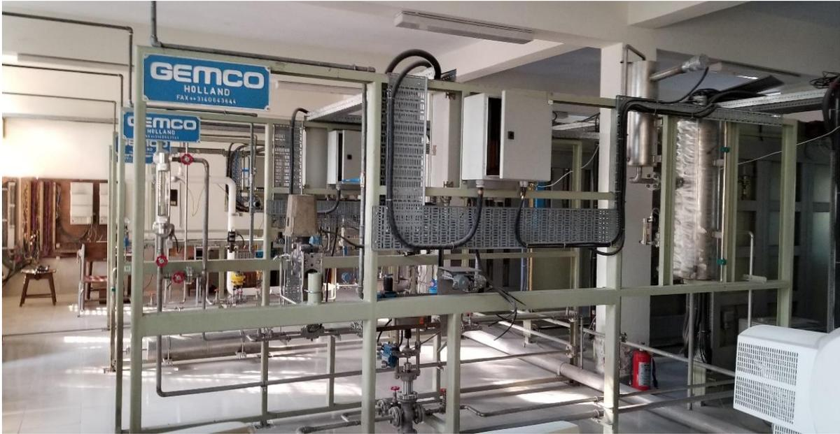
This lab is located at Ground floor of Academic Building-2. DCS Pilot plant is a fully computerized system incorporating practical facilities on computerized process control and automatic startup shutdown logic interlock widely used in industries.
