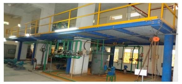
Here have the facility for a single stream heat exchange plant incorporating centrifugal pump, reciprocating pump, gear pump, vane pump, diaphragm pump, vessels and heat exchangers, different types of pipes & pipe fittings.
