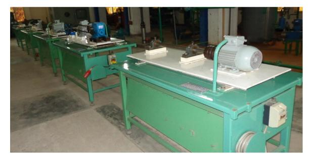
In this shop all methods of alignment technology are practiced i.e. gear alignment technique, both rigid & flexible coupling alignment, chain & sprocket, belt & pulley, machine train by precision & non- precision alignment methods.
